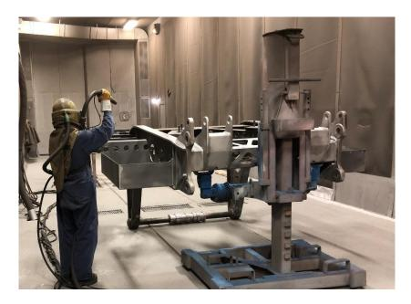
A large electrical and air source atomizes the aluminum and zinc metal into a spray. This spray travels to the metal surface where it instantaneously solidifies when it contacts the cool metal. The two metals are now mechanically boned together.
