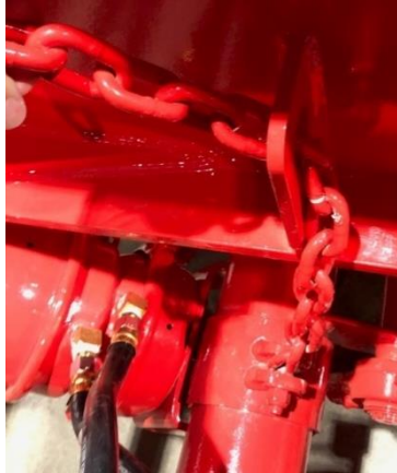
Air ride dumped; chain pulled to engage the shortest length
