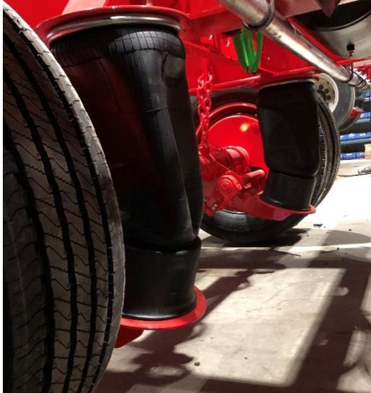
Collapsed air bag when trailer is lifted
