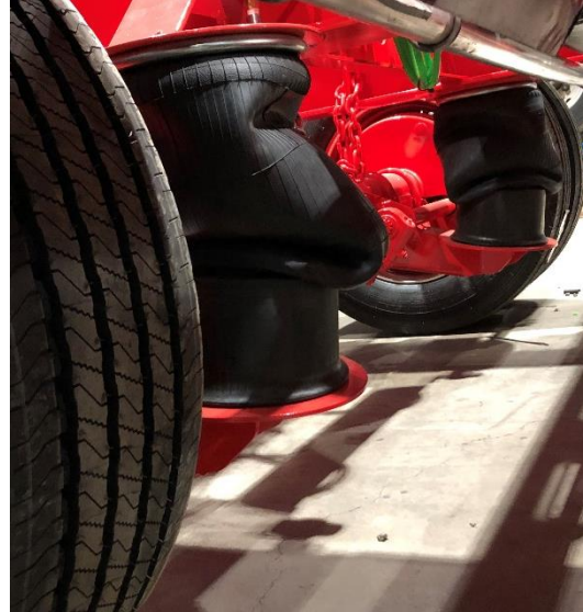
Air bag is folded onto itself when suspension is lowered
